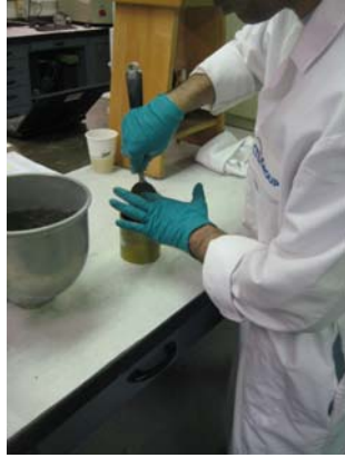
1. Place Mortar in Three Equal Layers
