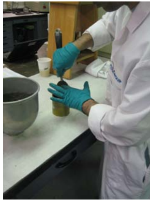
1. Place Mortar in Three Equal Layers
