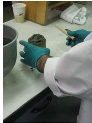
3. Tap the Sides of the Measure at Five Different Points.
