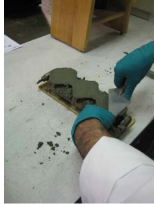
5. Draw Flat Side of Trowel Lightly Down Length of Mold.
