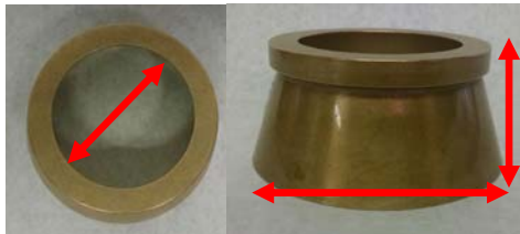
Diameter Top: 70 \pm 0.5 mm Diameter Bottom: 100 \pm 0.5 mm Height: 50 \pm 0.5 mm
