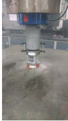
5. Center Specimen below Upper loading Block. Apply Load to True Plane Surfaces.
