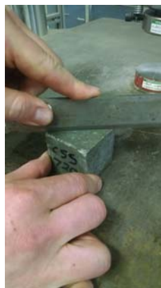
2. Check the Faces by Applying Straightedge.
