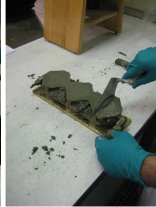
6. Cut off Mortar By Drawing Trowel with A Sawing Motion.
