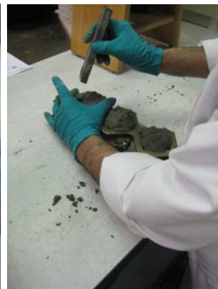
3. Fill Mold, Tamp as Specified, and Bring in Forced out Mortar.
