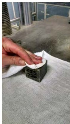
1. Wipe Specimen to SSD and Remove Loose Grains.
