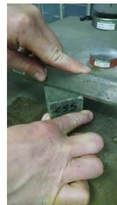
3. Note: If there is any Appreciable Curvature, Grind the faces.
