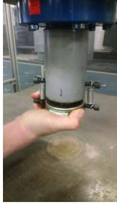
4. Check Spherical Seating Block is Free to Tilt.
