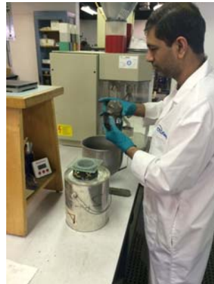
3. Press Ball in Larger End of Conical Ring
