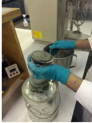
4. Place Conical Ring on Base Plate
