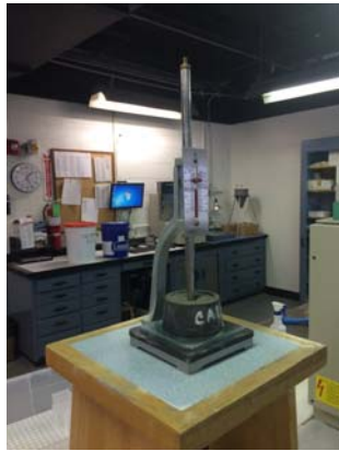
1. Center Ring and Base Plate under Rod
