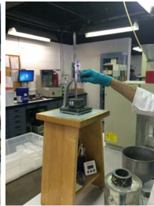
3. Release the Plunger. Time not Exceeding 30s after Mixing.
