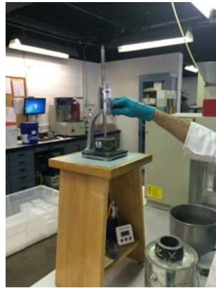
2. Place Plunger in Contact with Paste and Zero Reading
