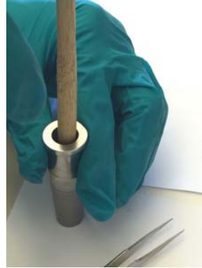
3. Press Edges Down with Rod
