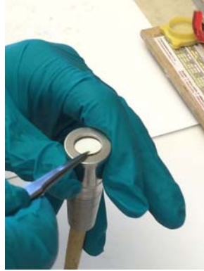
2. Place Filter Paper on Metal Disc
