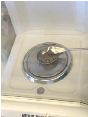
4. Measure Cement Mass to Nearest 0.001g
