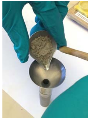
5. Place Cement Sample in Cell
